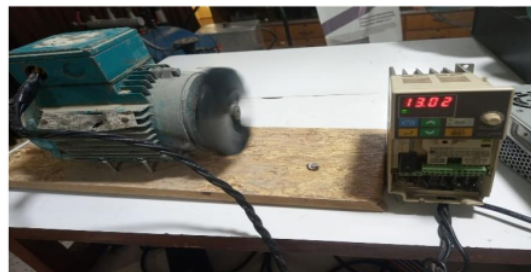
Figure 3-3 Induction motor with vfd Diagram
