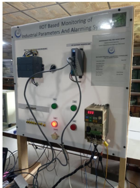
Figure 3-7 IOT Gateway with s7-1200
